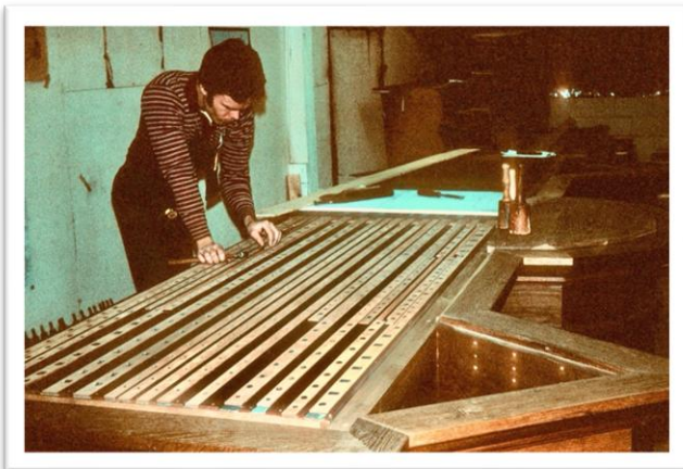
Michael Bigelow installs the sliders, which the stops move under the rows of pipes to stop or allow air up into the pipes so they speak.
